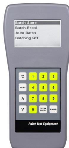
Multiple batches can be stored to a maximum of 10,000 readings.
