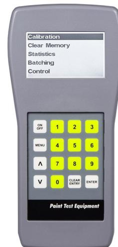
To exit from the menu, press the Menu button again and the Coating Thickness Meter will revert back to normal measurement mode.
