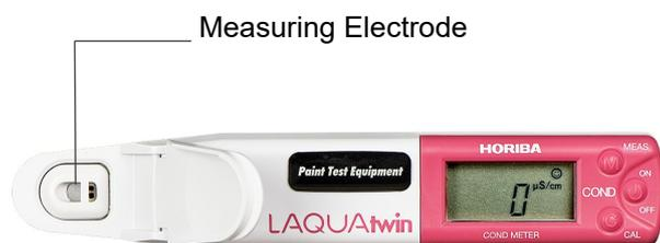
If the Measuring Electrode has not been used for a long period of time, or if the Electrode has been left extremely dry, then use this moistening procedure.
