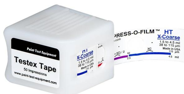
During compression the foam acquires an impression of the surface against which it is burnished. The highest peaks on the test surface displace the fully compressed foam and come to rest against the polyester substrate. The deepest valleys on the test surface create the highest peaks on the replica.
